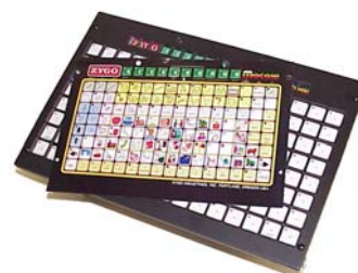
The DACTyl MACAW is a Green MACAW with a large keyboard — for those who need 128 larger-sized keys.
